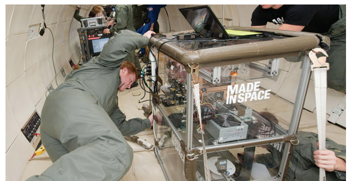
A 3D printer was installed aboard the International Space Station (ISS) in 2014 after the custom-built device passed final NASA certification. Having a 3D printer will enable astronauts to manufacture solutions to unforeseen problems, without having to wait for a resupply mission.
