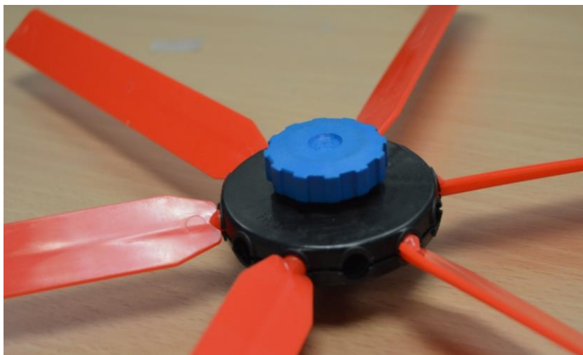
Figure 2. These blades have been set into the hub at the same angle ( 45^{\circ} ).
