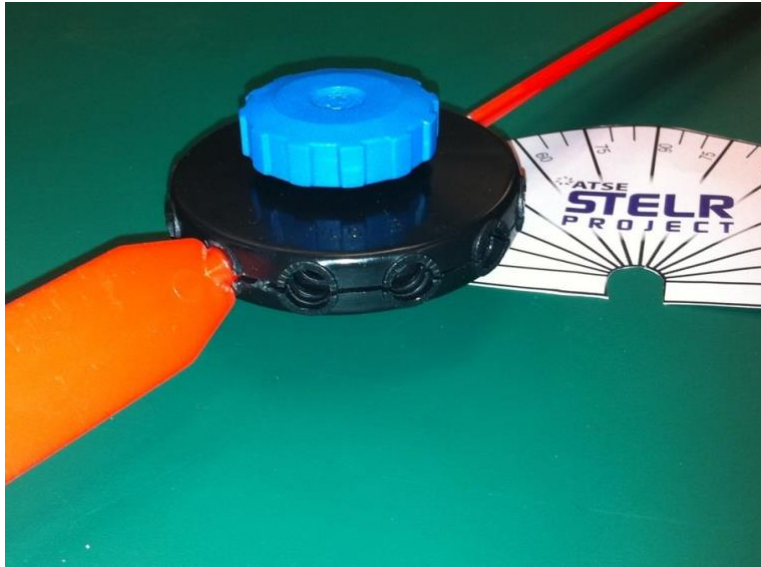
Figure 2. These blades have been set into the hub at the same angle ( 45^{\circ} ).
